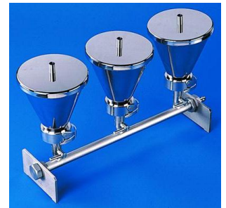
Figure 1 – Rampe de filtration
